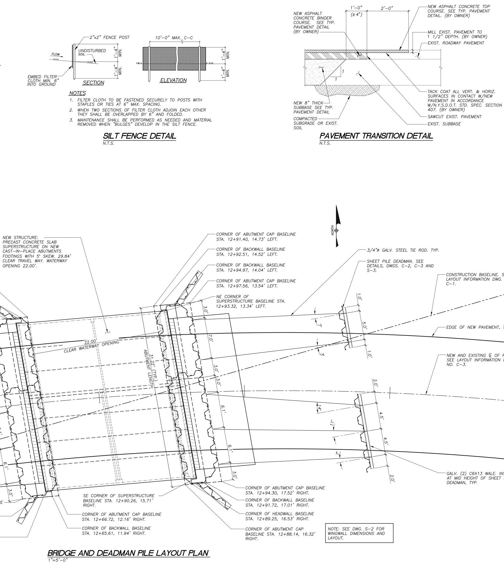
CONSTRUCTION BASELINE. SEE LAYOUT INFORMATION DWG. NO. — NEW AND EXISTING ♀ OF ROAD. SEE LAYOUT INFORMATION DWG. — GALV. (2) C6X13 WALE. INSTALL AT MID HEIGHT OF SHEET PILE DEADMAN, TYP.
