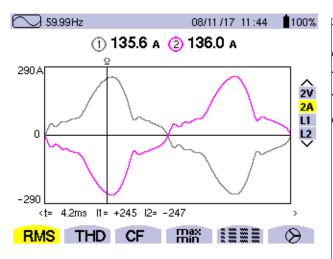
This is the typical current waveform with the 2 commercial radio transmitters operating on utility power. Note the high level of distortion.
