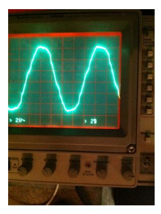
IMG\_1959 is a voltmeter picture of the voltage supplied to the panel while on Utility.
