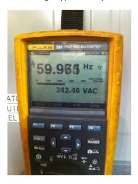
IMG\_1947 is the waveform of the voltage from the generator with no load.
