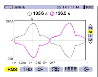
This is the typical current waveform with the 2 commercial radio transmitters operating on utility power. Note
