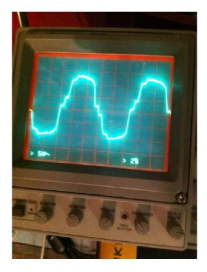
IMG\_1944 is a voltmeter picture of the voltage supplied to the panel while on Generator.
