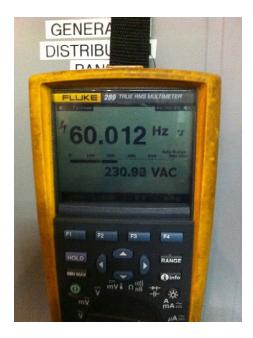
IMG\_1941 is the waveform of the voltage coming out of the generators ATS on Generator and feeding the breaker panel.
