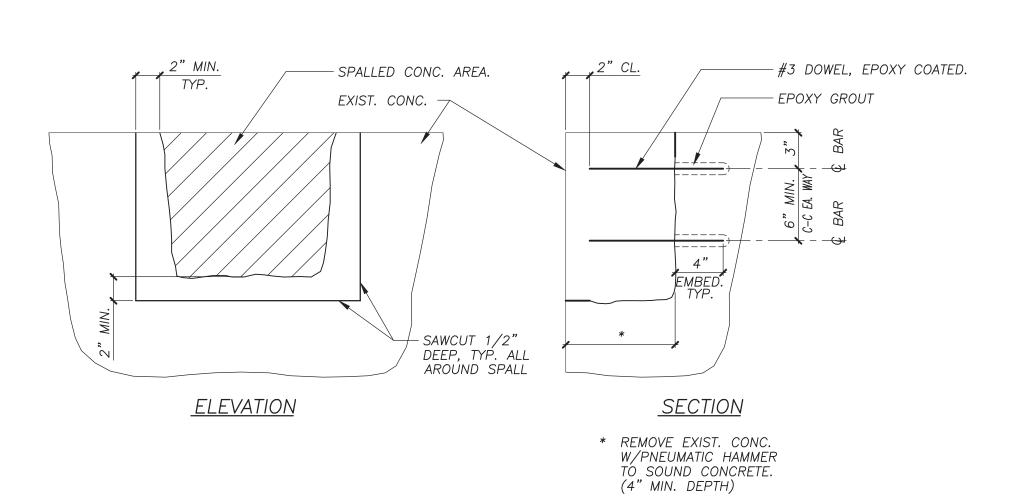
TYPICAL SPALLED CONCRETE REPAIR DETAIL
