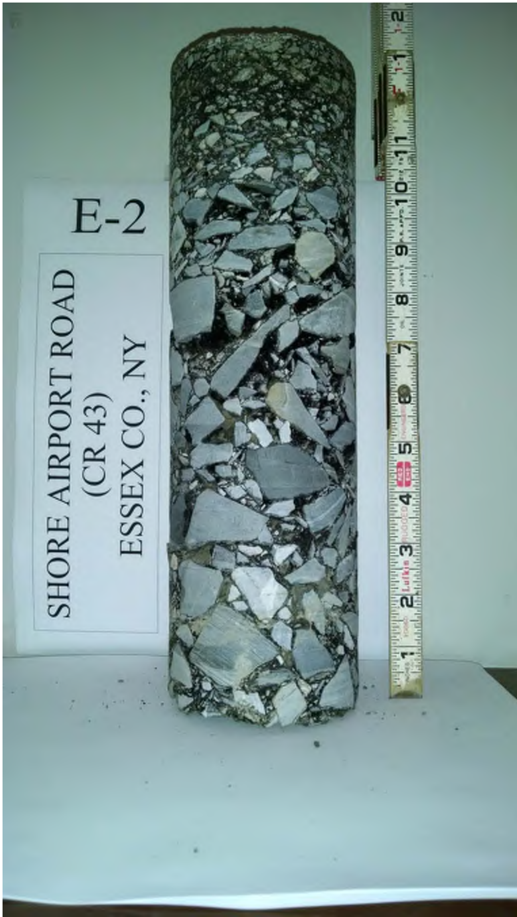
Pavement core at E-2 (in southbound travel lane)
