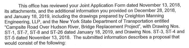
The discharge of fill material into waters of the United States to facilitate the replacement of a bridge carrying Campsite Road over the Hudson River. The existing bridge would be replaced on the same horizontal alignment with a bridge having a span of approximately 100 feet and an out to out width of 27'4".
