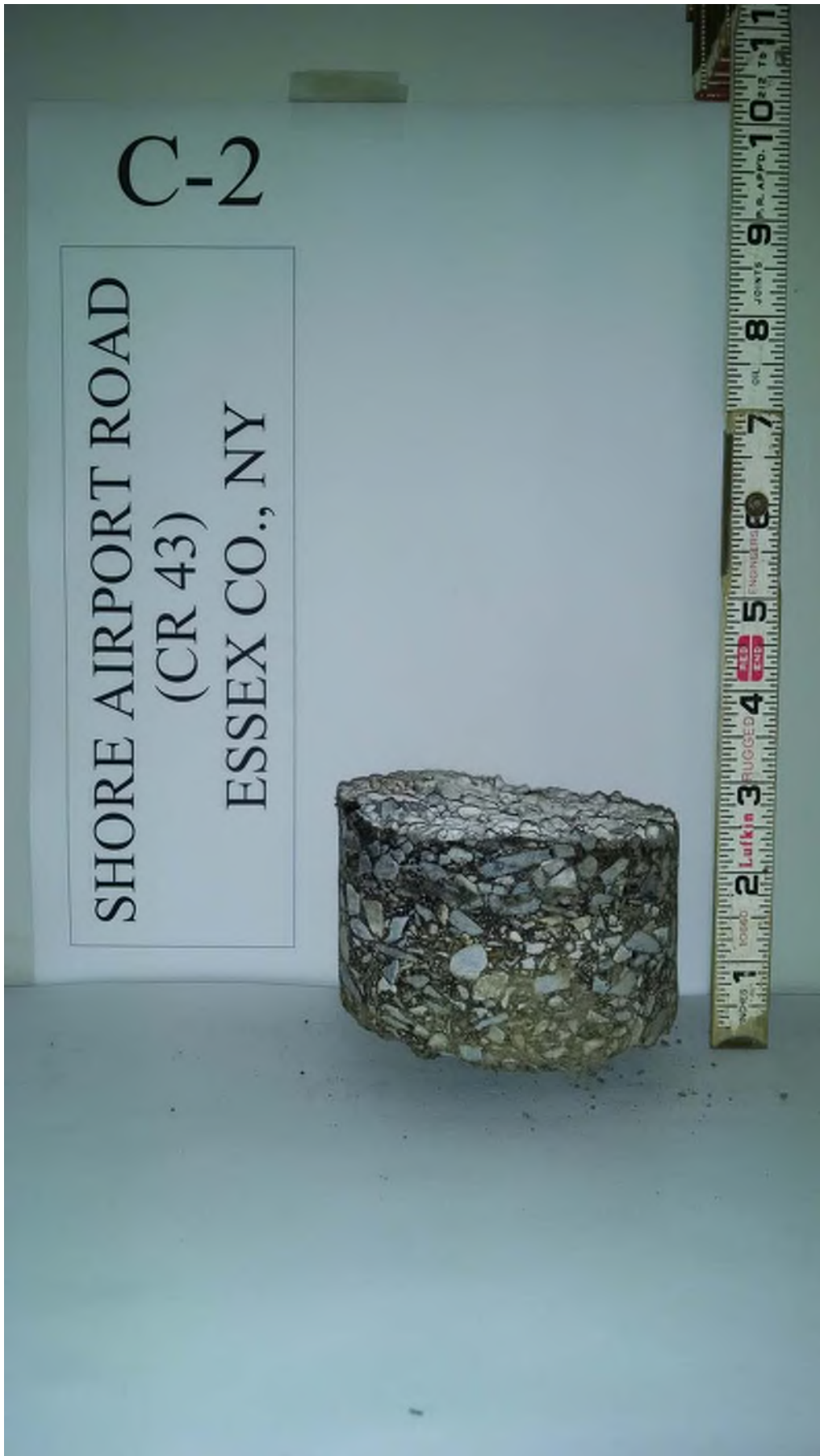
Pavement core at C-2 (in northbound shoulder)
