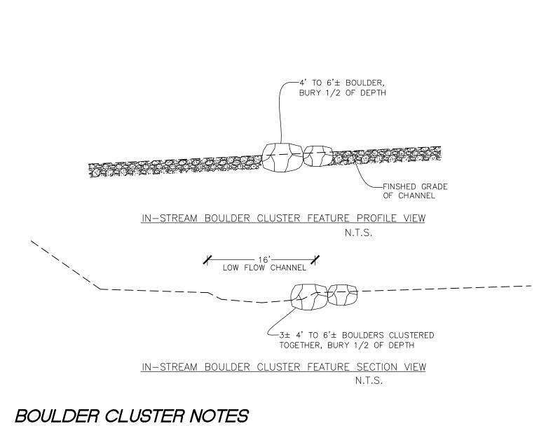
1) BOULDERS MUST BE APPROVED, HARD, ANGULAR, BLASTED, STRONG, RESISTANT TO WEATHERING, AND RING WHEN
