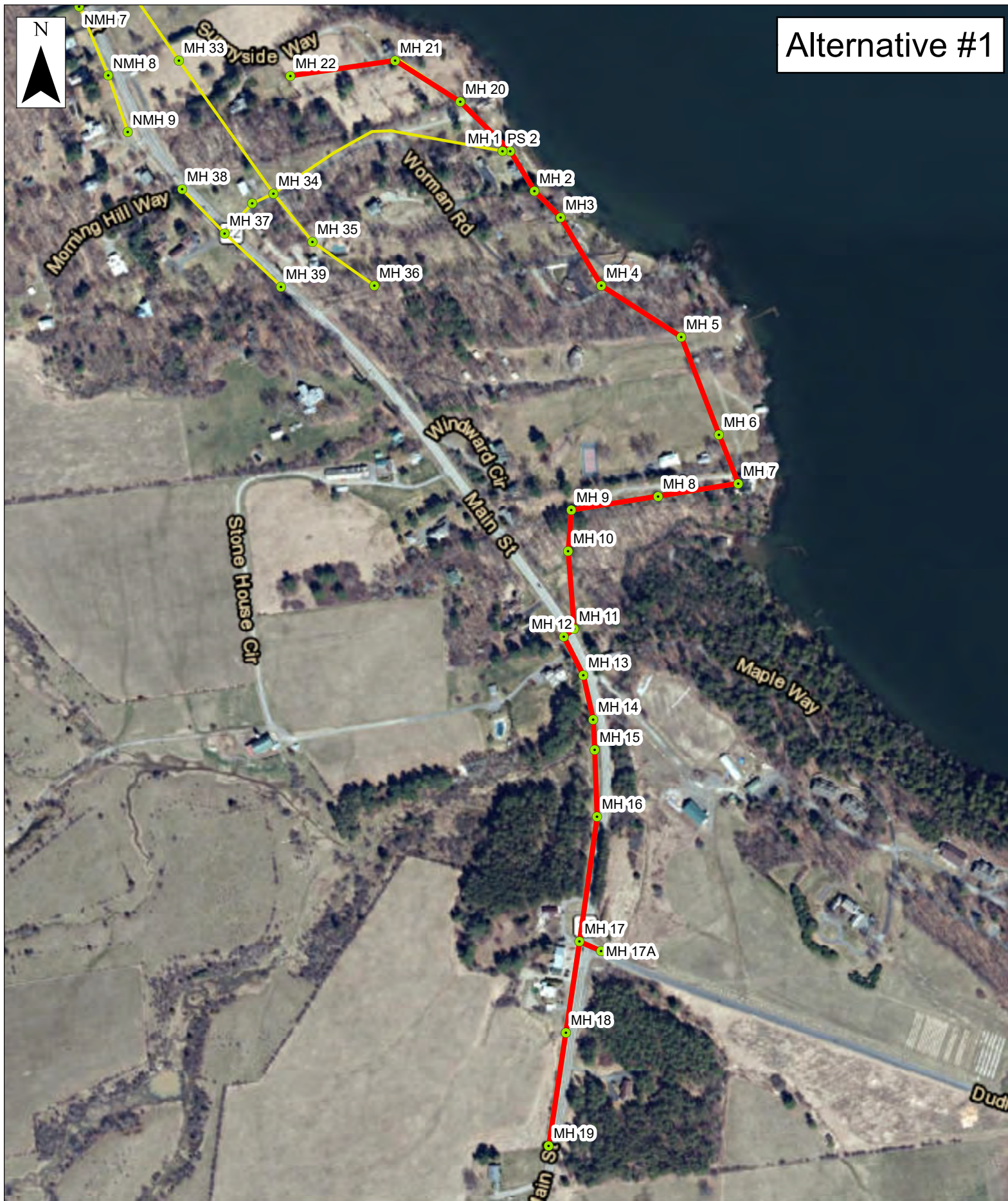
Figure 3.10.2: Pump Station #2 & Worman Road Alternatives Sewer Service Section Around the Worman Road Pump Station #2
