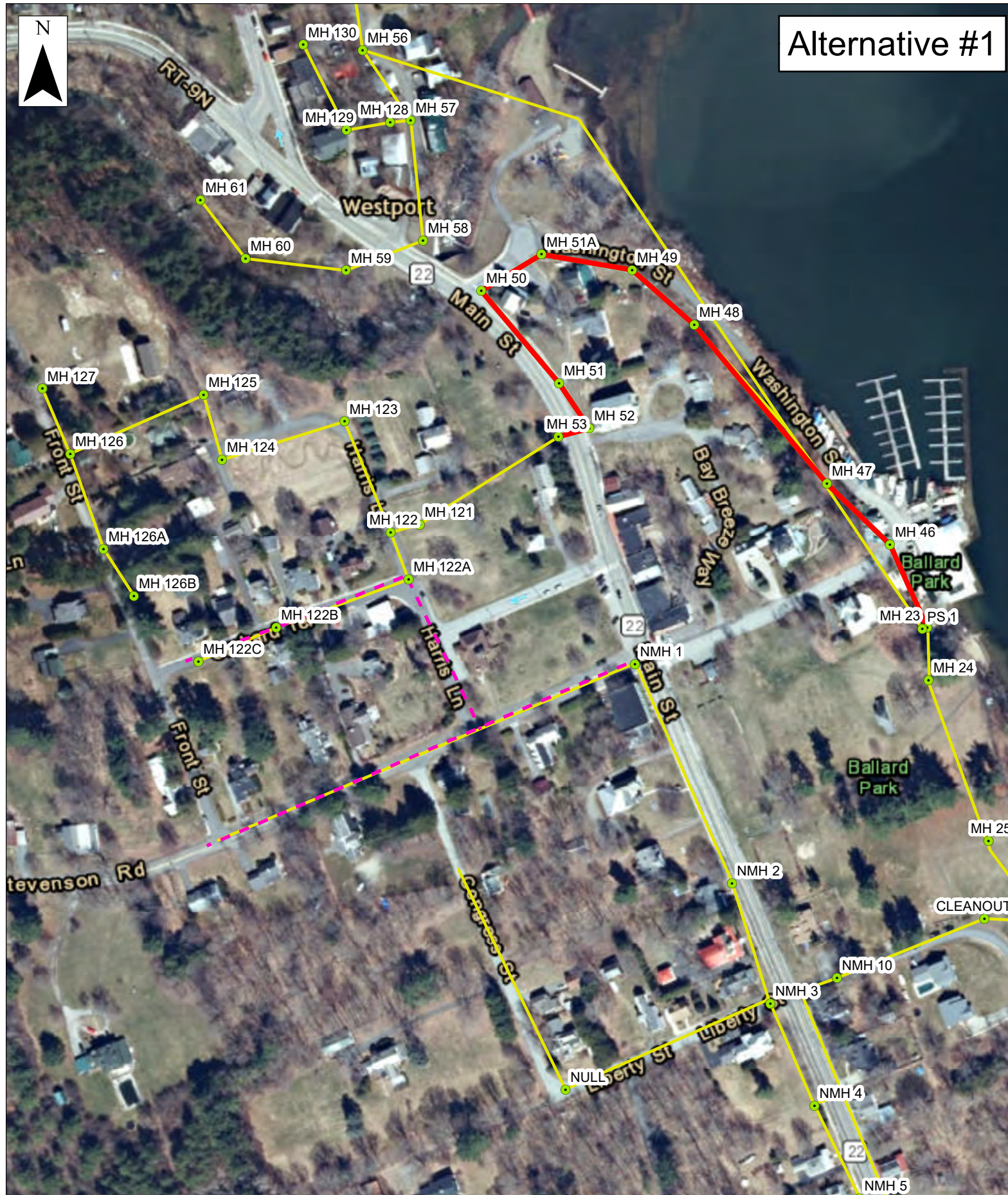
Figure 3.10.8: Harris Lane Alternatives Sewer Service Section Around Harris Lane and Washington Street
