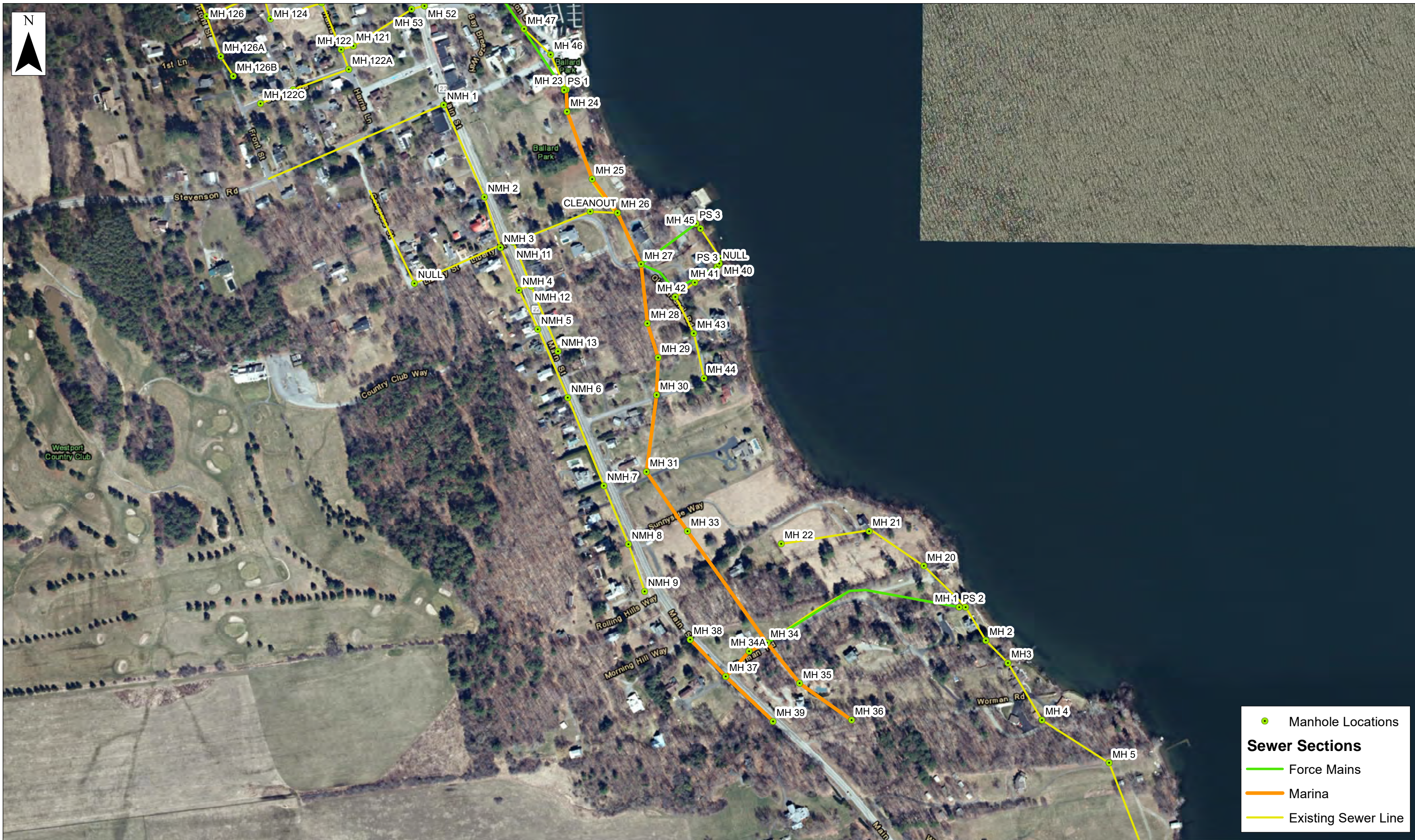
Figure 2.4.8: Pump Station #1 Service Area Sewer Service Section Around the Marina Pump Station #1
