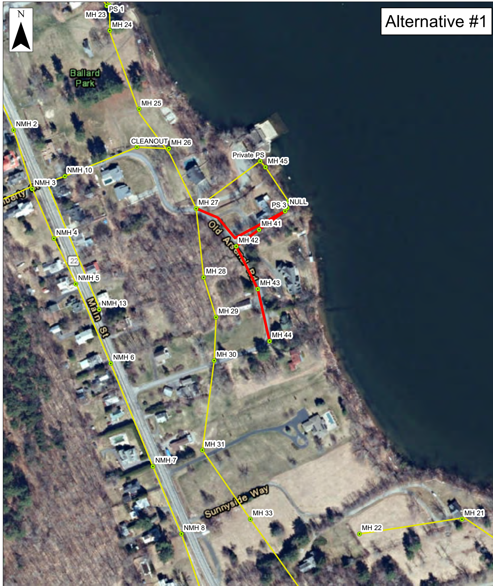
Figure 3.10.3: Pump Station #3 & Old Arsenal Road Alternatives Sewer Service Section Around Old Arsenal Road Pump Station #3
