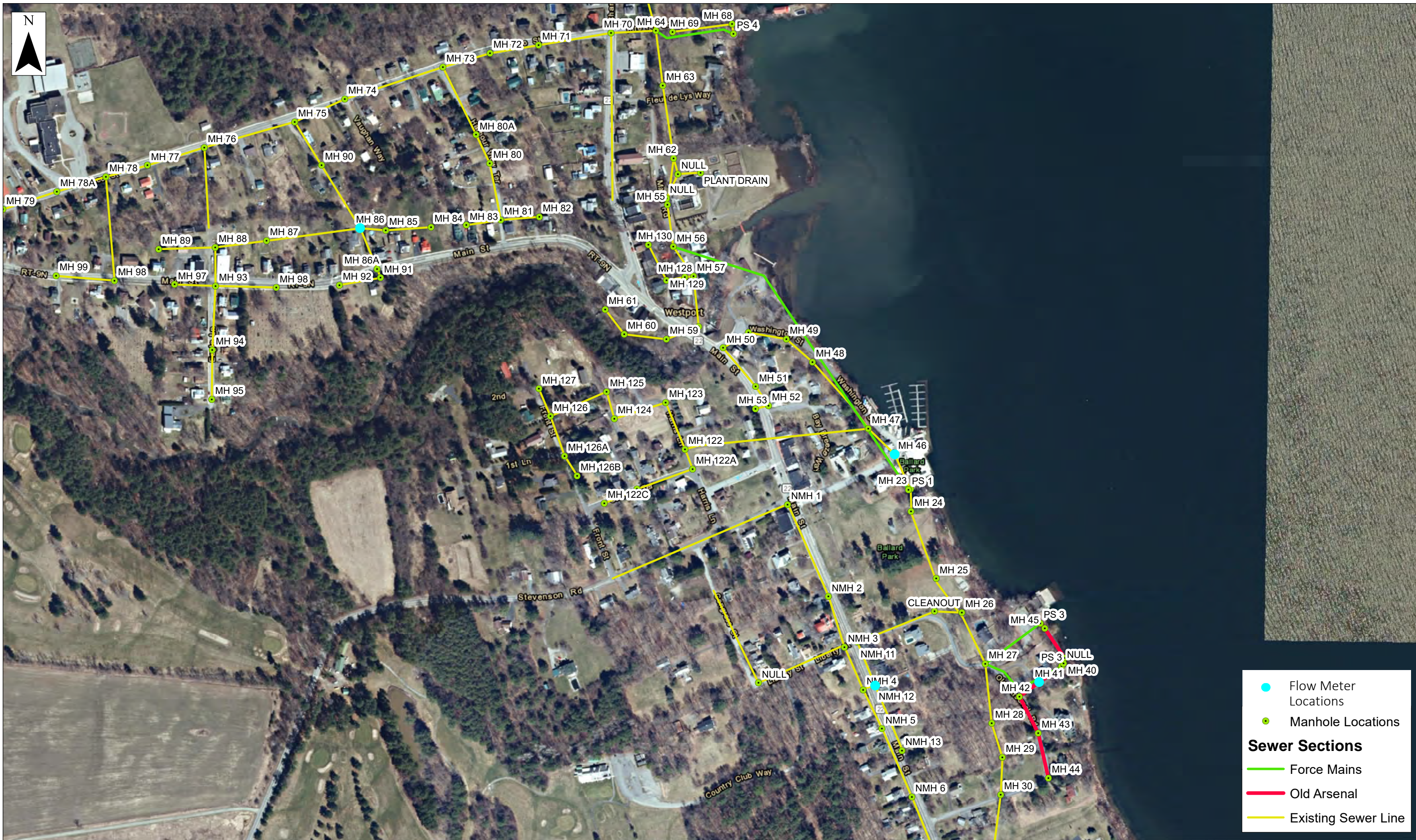
Figure 2.4.1A: Flow Meter Locations Highlighted Manholes where Flow Meters Were Installed
