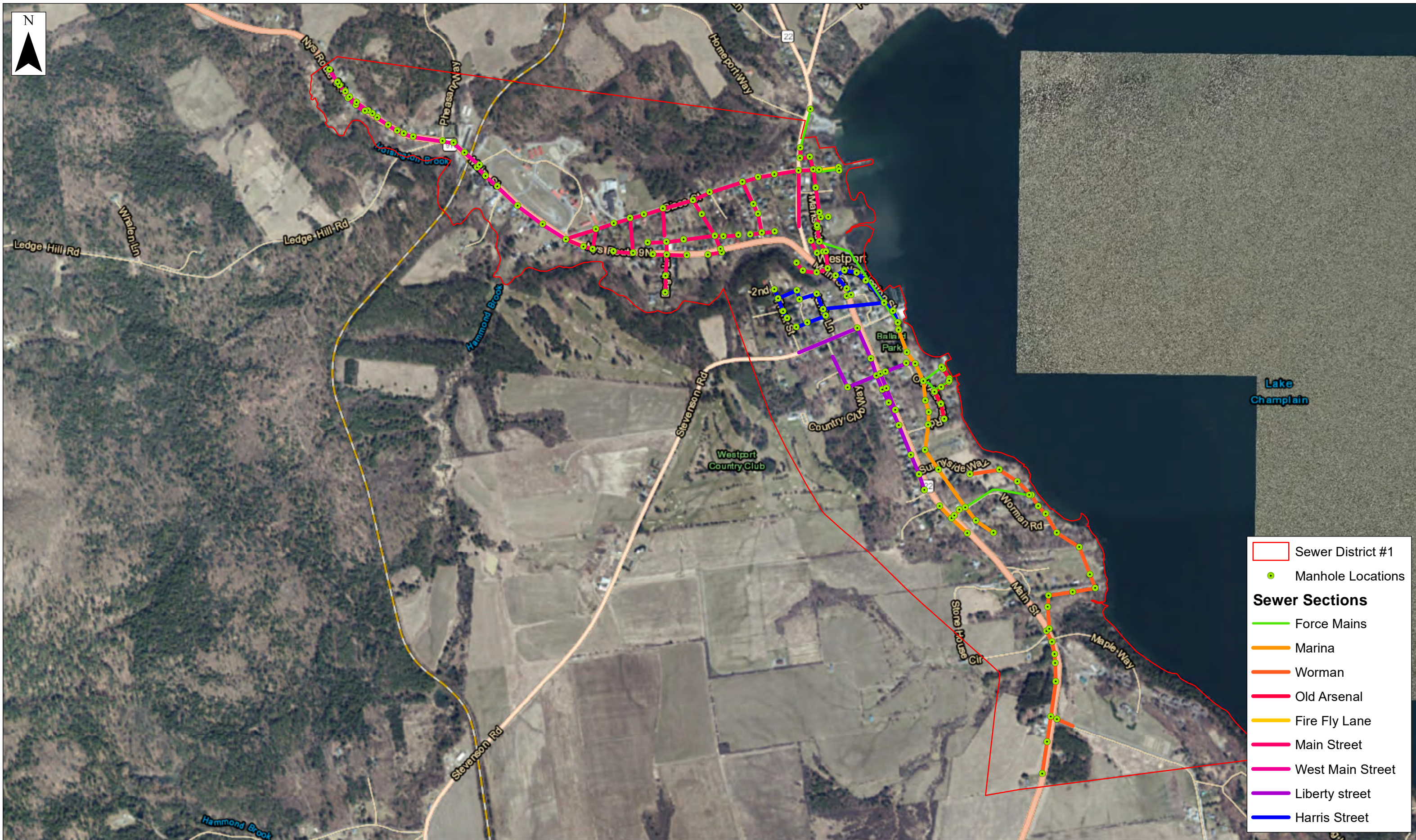
Figure 2.4.7 Existing Sewer Sewer Based on Manhole Collection and Historic Maps
