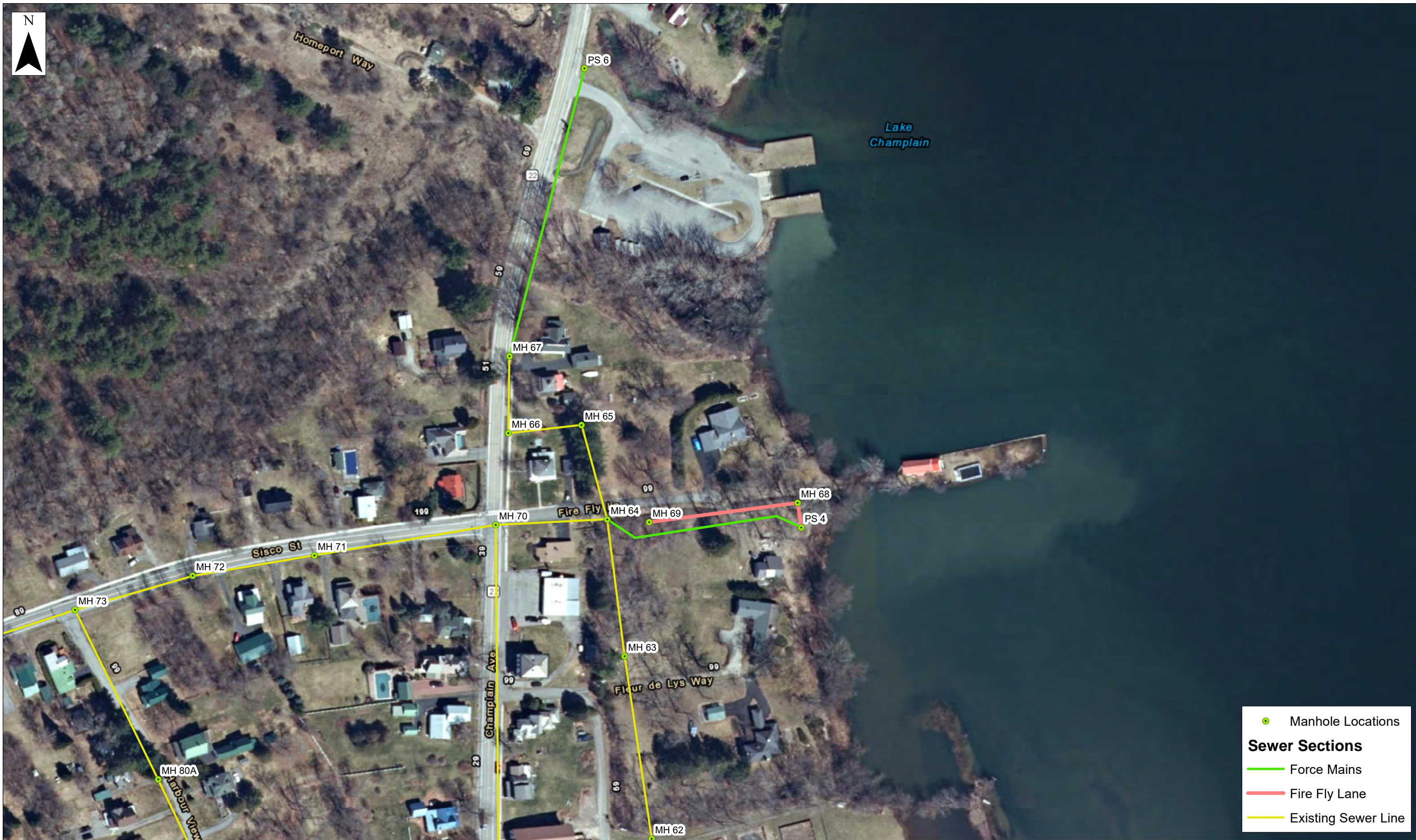
Figure 2.4.11: Pump Station #4 Service Area Sewer Service Section Around Fire Fly Lane Pump Station #4
