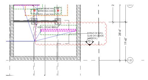
The dashed green line (around the pink dashed line) indicates a new reinforced concrete footing for the new shearwall. The existing slab would need to be cut out for the new footing to be installed. The typical shearwall sections would apply. See 'SN18' note and sections.
